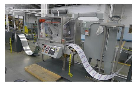
Figure 5. Image of the aluminum straightening and reflective sheeting application process.
