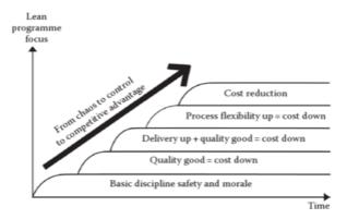
Figure 1. Lean improvement stages. Reprinted from The Green Factory: Creating Lean and Sustainable Manufacturing (9), by A. Pampanelli, N. Trivedi, & P. Found, 2015. Copyright 2015 by Productivity Press.
